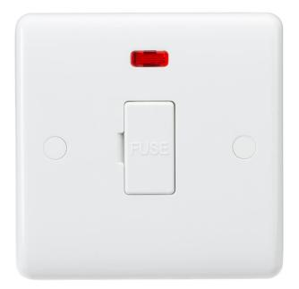
Fused spur units or connection units are an electrical switch with a built in fuse, designed for appliances that do not have or require a fused plug top. Fused spur units are also used for high powered electrical equipment with heavy continuous load, so that the appliance can be isolated by a single cable from a ring main for safety and maintenance purposes. 13A rated available with and without a double pole switch/neon.
